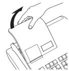
**2** Remove the battery compartment cover.
