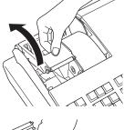
**4** Put the leading end of the paper over the printer.
