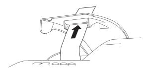
9. Reposition, close and lock the printer compartment cover.
