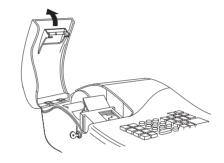
2. Lift the paper journal winder spindle out of the printer compartment.
