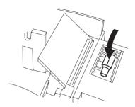
4. Reposition, close and lock the printer compartment cover.
