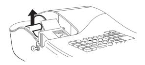
3. Remove the battery compartment cover by pressing on the arrow impressed on the cover and lifting upwards, as shown by the arrows in the figure.
