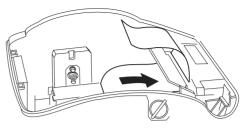
Set the control switch to R1 or R2, press the [Feed] key and manually feed the paper into the slot until the paper catches and advances approximately six to ten inches above the print mechanism.
