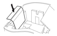
7. Reposition the journal winder spindle, then reposition, close and lock the printer compartment cover.
