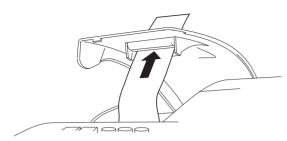
9. Reposition, close and lock the printer compartment cover.
