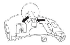
8. Pass the edge of the customer receipt through the receipt window on the compartment cover.
