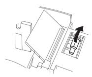
3. To install a new ink roller, insert the ink roller according to the markings "L" (Left) and "R" (Right) by pressing downward to lock it into position.
