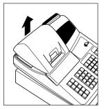
The printer is one station type thermal printer, and therefore it does not require any type of ink ribbon or cartridge.
