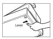
The drawer automatically opens. However, when a power failure occurs or the machine becomes out of order, slide the lever located on the bottom of the machine in the direction of the arrow. (See the diagram at the left.) The drawer will not open if it is locked with the key.
