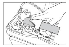
6. While holding down the paper, slowly close the print roller arm, and push down the arm until you hear a click locking the arm. Make sure securely you push down the center of the wing part of the arm as per the diagram. The paper will be fed automatically.
