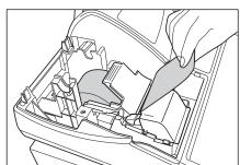
replace the printer cover. Press the ↑ key to make sure the paper end comes out of the printer cover and clean paper appears. If the paper end does not come out, open the printer
