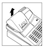
The printer is one station type thermal printer, and therefore it does not require any type of ink ribbon or cartridge.
