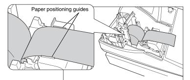
4. While holding down the paper, slowly close the print roller arm, and push down the arm until you hear a click locking the arm. Make sure securely you push down the center of the wing part of the arm as per the diagram. The paper will be fed automatically.
